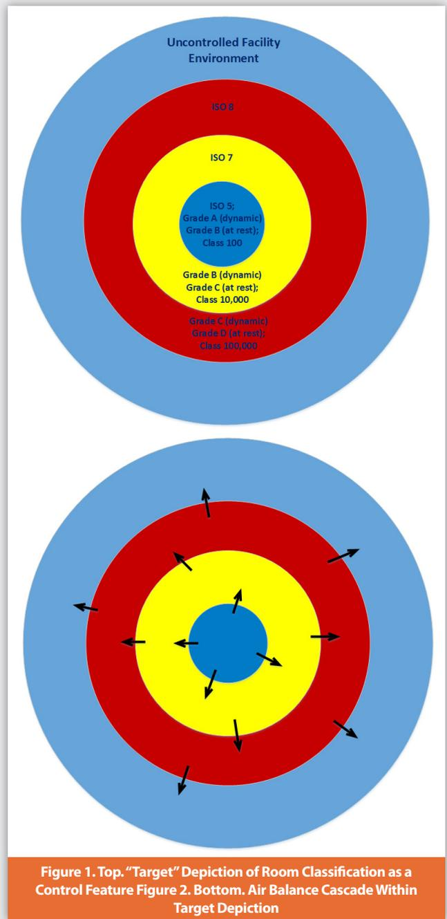
**Figure 1. Top. “Target” Depiction of Room Classification as a Control Feature Figure 2. Bottom. Air Balance Cascade Within Target Depiction**
